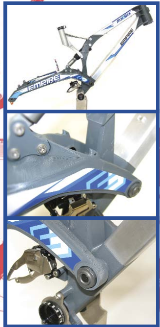
Figures 2, 3 & 4. Closeups of the 3D printed components integrated with the extruded frame sections
